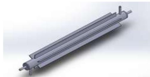
Fig. 2. External finned double pipe heat exchanger.
