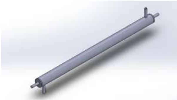
Fig. 3. Internal finned double pipe heat exchanger.
