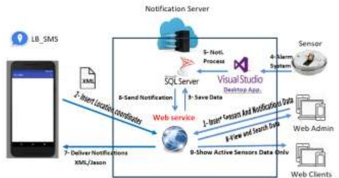
Fig. 5.1. LB\_SMS system components.
