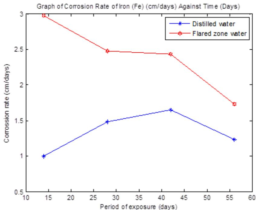
Fig. 2. Corrosion rate of Iron (Fe) soaked in distilled water and water from flared zone (Ogbogu gas flow station).
