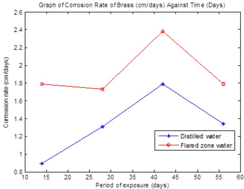
Fig. 1. Corrosion rate of Brass soaked in distilled water and water from flared zone (Ogbogu gas flow station).
