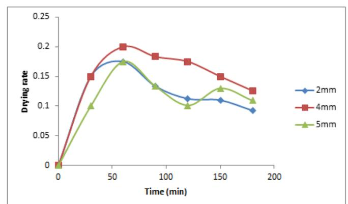
Fig. 5. Variation of drying rate with time under force convection.
