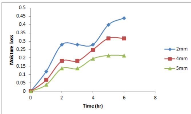
Fig. 1. Variation of moisture content with drying time under free convection.
