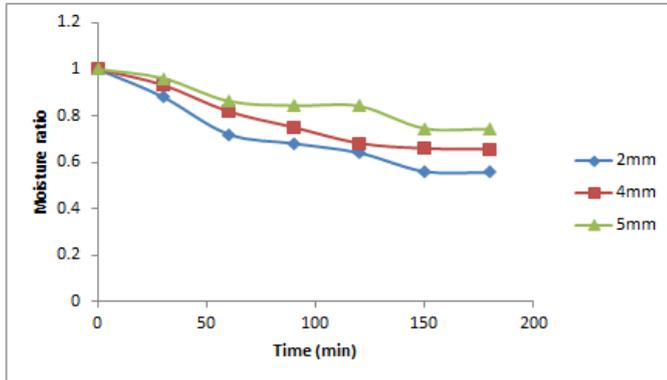
Fig. 6. Variation of moisture ratio with time under force convection.
