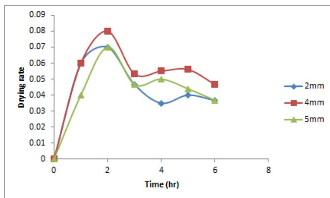
Fig. 2. Variation of drying rate with time under free convection
