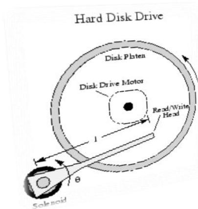
Fig. 2. Schematic diagram of a typical hard disk drive [13].
