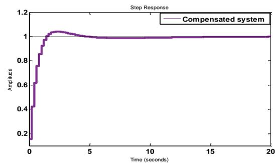
Fig. 6. Step response of compensated positioning system.
