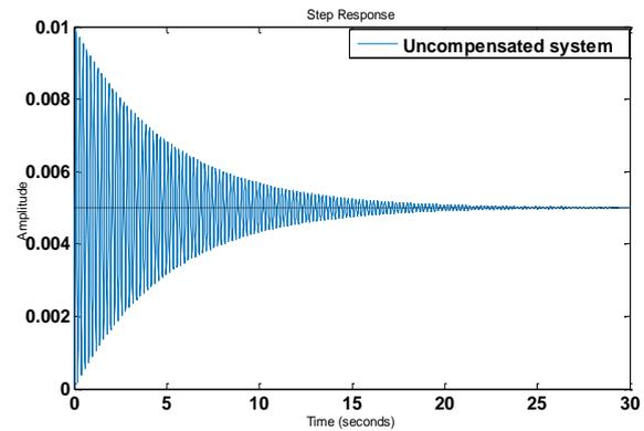
Fig. 5. Step response of uncompensated positioning system.
