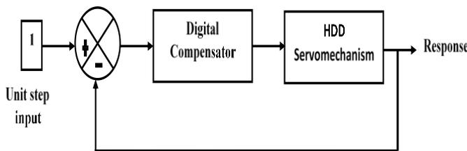
Fig. 3. System configuration.
