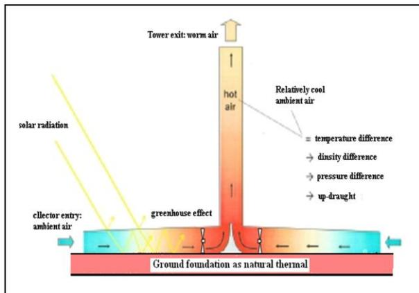
Fig. 1. Solar tower working principles
