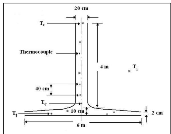
Fig. 2. Schematic diagram of the solar chimney and thermocouples distribution.
