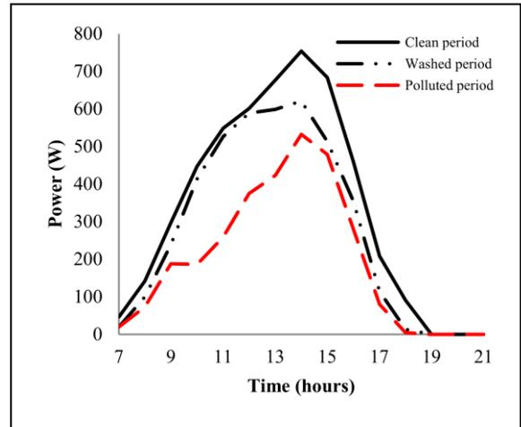
Fig. 7. The studied chimneys output powers distribution through the day
