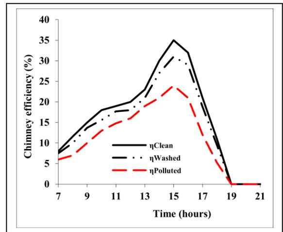
Fig. 8. The solar chimneys efficiencies distribution during the day
