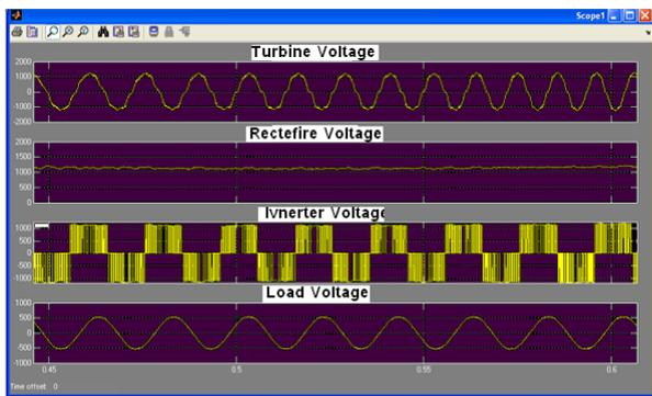
Fig. 2. Wind turbine performances with a synchronized 2MW power generator.
