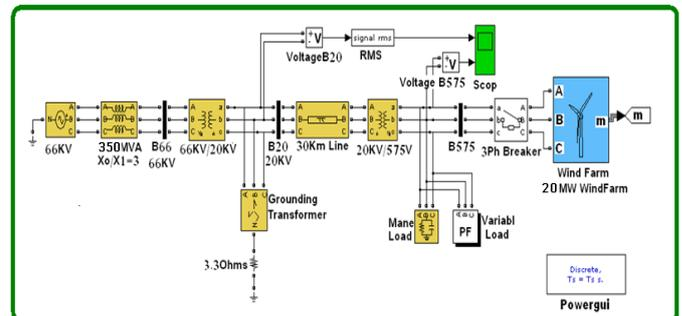
Fig. 3. Wind farm connected to an electric network using MATLAB-SIMULINK.
