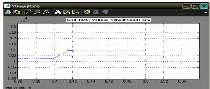
Fig. 4. Network voltage before 20MW wind farm connection.
