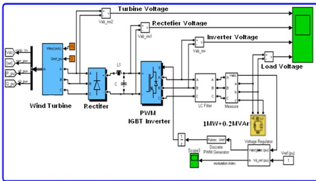
Fig. 1. Simulation of a 2MW synchronous generator wind turbine with electronic switches in Matlab-Simulink.
