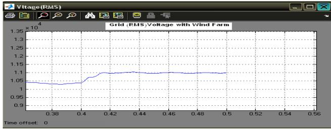
Fig. 5. Network voltages after the 20MW wind farm linkage.
