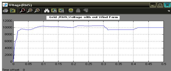
Fig. 6. Network voltages before 30MW wind farm connection.
