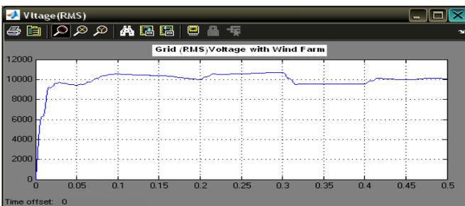
Fig. 7. Network voltages after the 30MW wind farm linkage.
