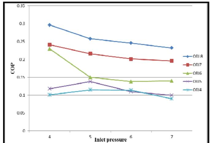
Fig. 4. Inlet pressure vs COP (From Aluminum material)
