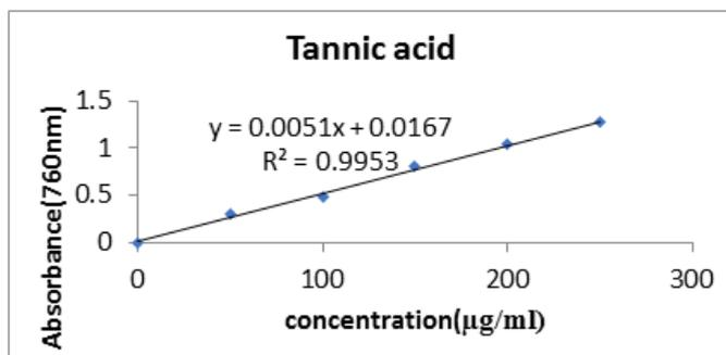
Fig. 3.2a. Standard calibration curve for total phenolic content for standard tannic acid.
