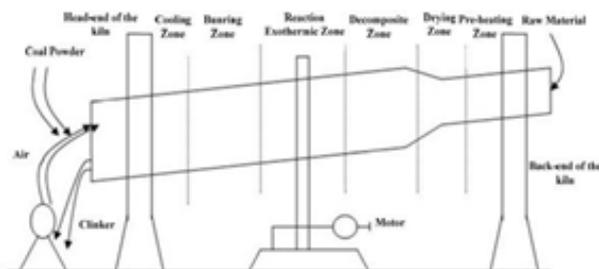
Fig. 1. Cement rotary kiln system.
