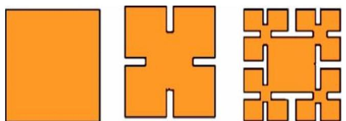
Fig. 3. Different iterations of minkowski fractal antenna.
