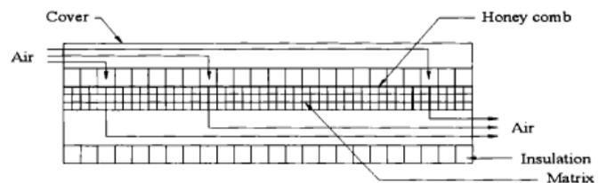
Honeycomb porous bed air heater
