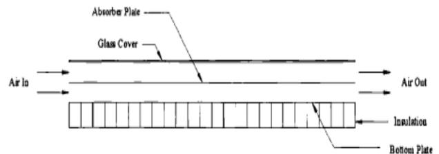
Type III Non-porous solar air heater (flow both above and beneath the absorber)
