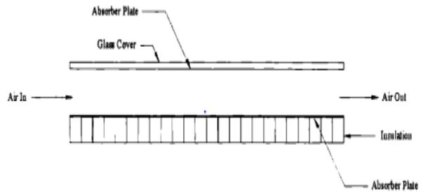
Type II Non-porous solar air heater (flow under the absorber)
