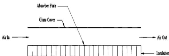
Type I Non-porous solar air heater (flow above the absorber)
