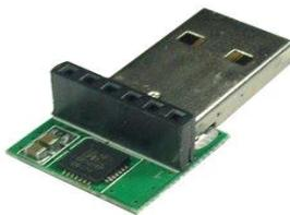
Fig. 4. USB to TTL converter.
