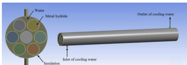
Fig. 3. The geometry of tank for simulation.
