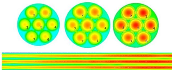
Fig. 6. Heat contours of the stack after the simulation has ended.
