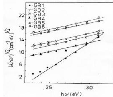
Fig. 2 . Plot of  $\alpha' hv$  versus  $hv$  for samples GB<sub>1</sub>, GB<sub>2</sub>, GB<sub>3</sub>, GB<sub>4</sub>, GB<sub>5</sub>, GB<sub>6</sub>.
