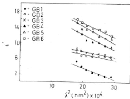
Fig. 3. Plot of optical dielectric constant  $\epsilon'$  versus  $\lambda'^2$  for six samples GB<sub>1</sub>, GB<sub>2</sub>, GB<sub>3</sub>, GB<sub>4</sub>, GB<sub>5</sub>, GB<sub>6</sub>.
