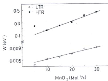
Fig. 6. Variation of activation energy (w) with  $\text{MnO}_2$  mol% in LTR and HTR for the glass samples.
