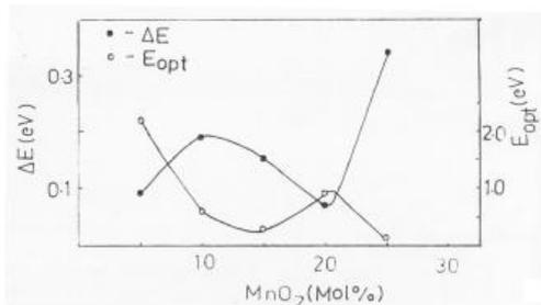
Fig. 4. Plot of optical energy gap  $E_{opt}$  and band tailing energy  $\Delta E$  versus mol% of  $MnO_2$  composition of six samples.
