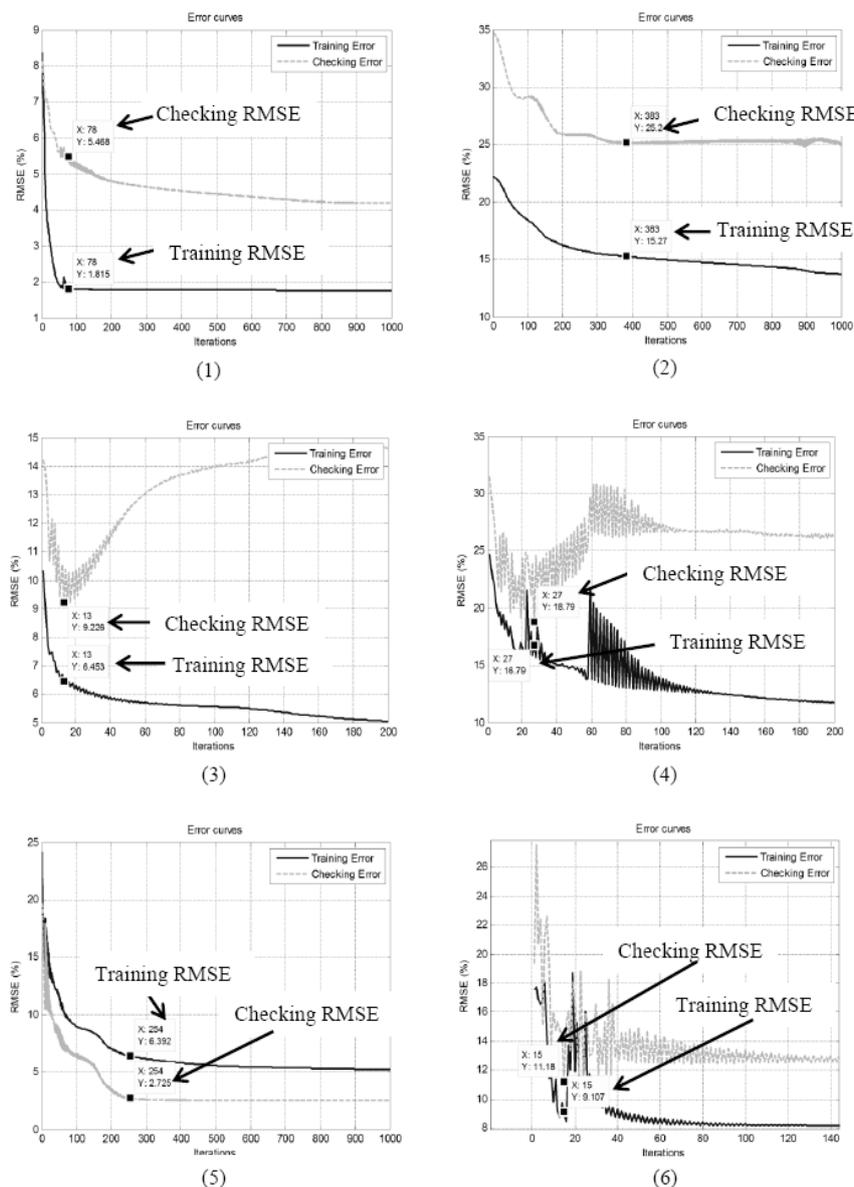
Fig. 5. Trial 1 RMSE training and checking curves for the six ANFIS.
