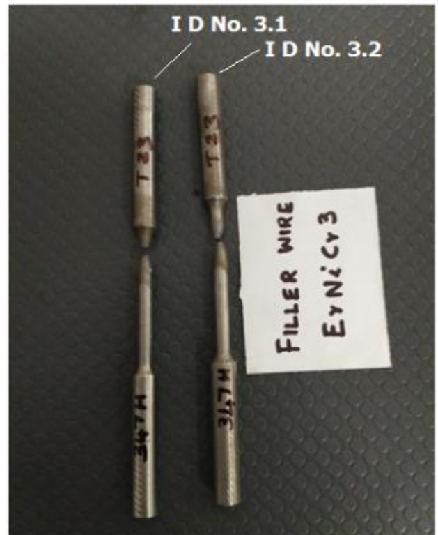
Fig. 6. Tensile tested specimen welded with ErNiCr3 filler wire.
