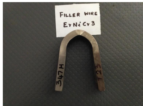
Fig. 3. Bend specimen welded with ErNiCr3 filler wire.
