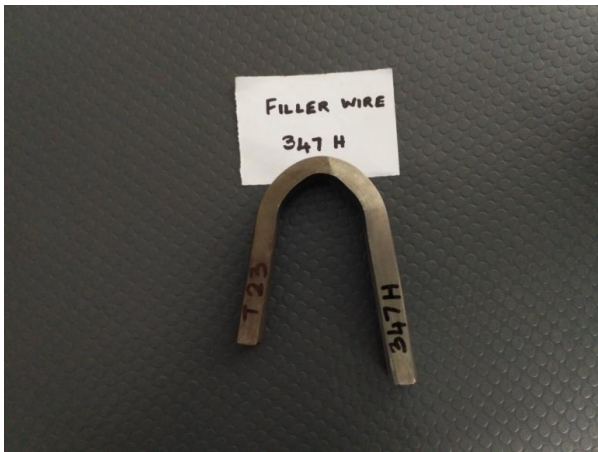
Fig. 4. Bend specimen welded with 347H filler wire.
