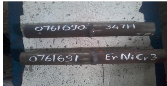
Fig. 1. Welded specimen (T23+SS 347H) with 347 H (joint no.0761690) and ERNiCr3 (joint no. 0761691) filler wire.
