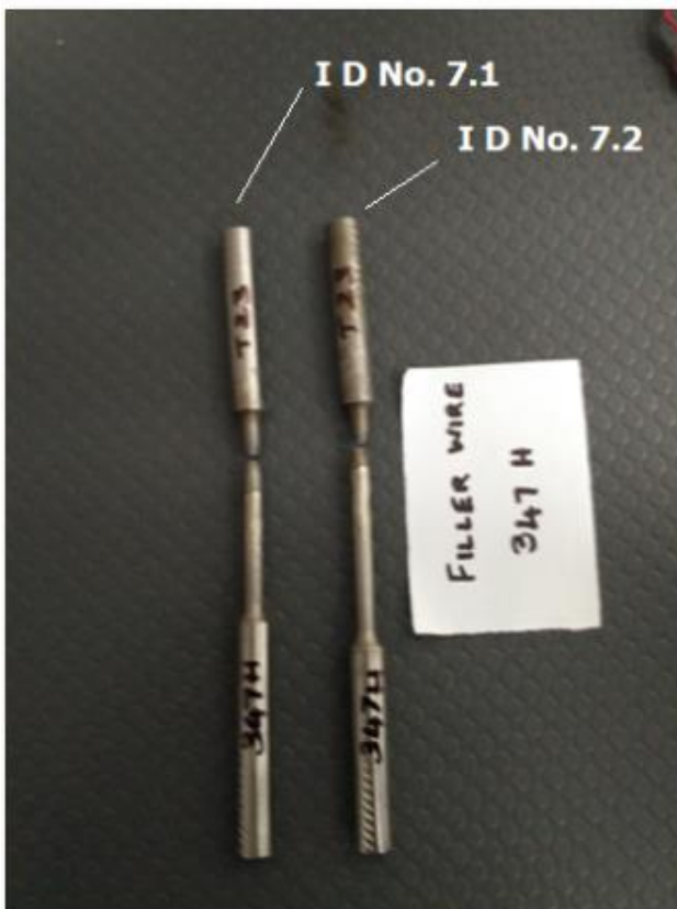
Fig. 5. Tensile tested specimen welded with 347H filler wire.
