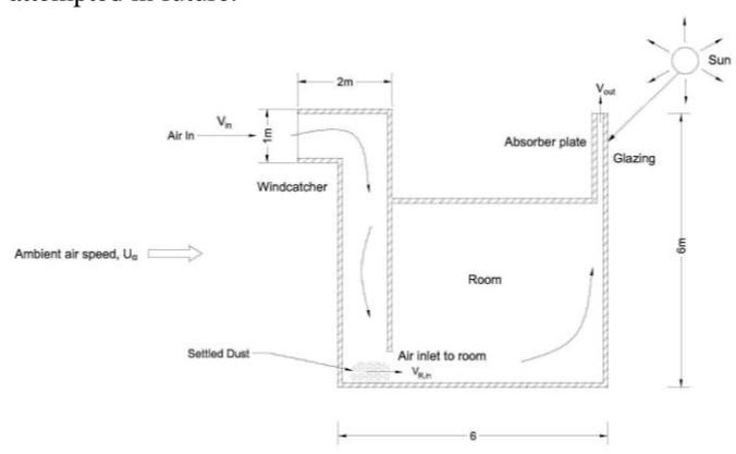
Fig. 1. A simple combinatorial wind catcher-solar chimney system.
