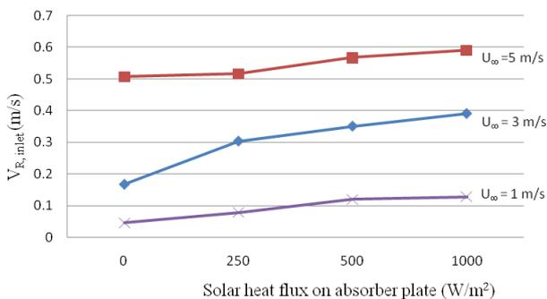
Fig. 7. Variation of room inlet air velocity with chimney effect.
