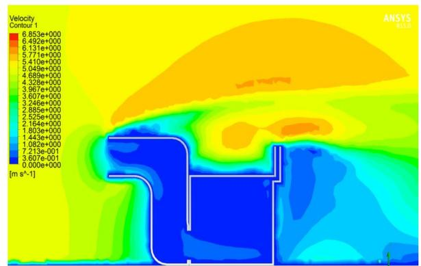
Fig. 12. Velocity contours for air flow with changed wind catcher geometry, and no heat flux (effect of wind catcher alone);  $U_{\infty} = 5$  m/s.
