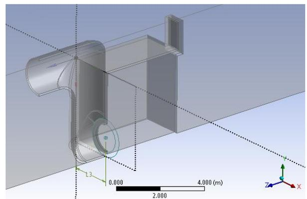
Fig. 11. Change in windcatcher geometry (rectangular to circular cross section, area remaining the same).
