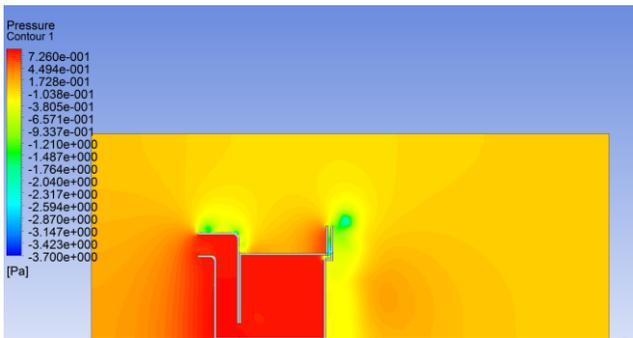
Fig. 6. Pressure contours for airflow ( $U_\infty = 1$  m/s, heat flux  $E = 250$  W/m<sup>2</sup>).
