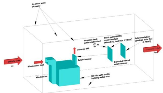
Fig. 2. Boundary conditions for simulations on the combinatorial system.
