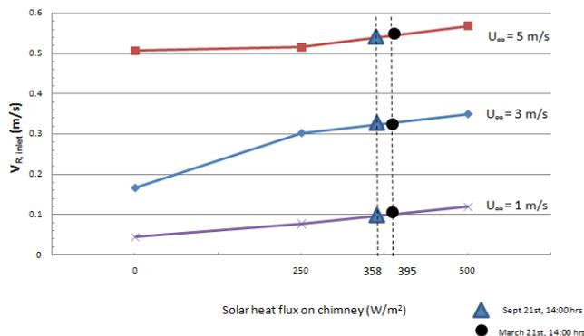
Fig. 10. Seasonal performance of the combinatorial system for two specified days in a year (interpolation method).
