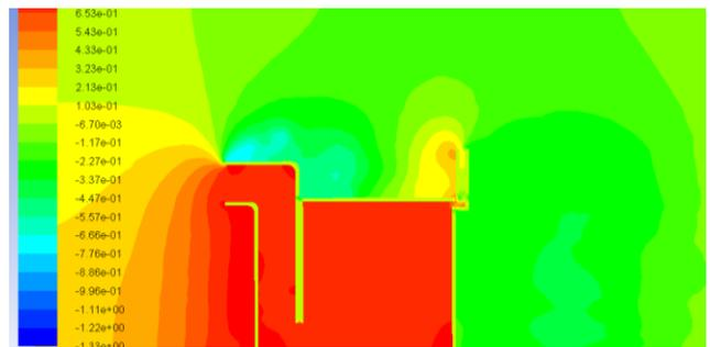
Fig. 4. Pressure contours vectors for airflow ( $U_\infty = 1$  m/s, no heat flux).
