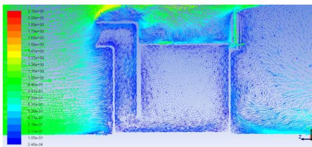
Fig. 3. Velocity vectors for airflow ( $U_\infty = 1$  m/s, no heat flux)
