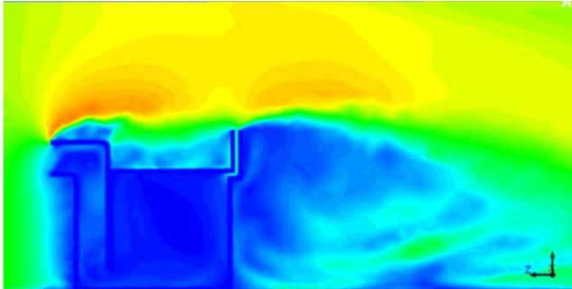
Fig. 5. Velocity contours for airflow ( $U_\infty = 1$  m/s, heat flux  $E = 250$  W/m<sup>2</sup>).
