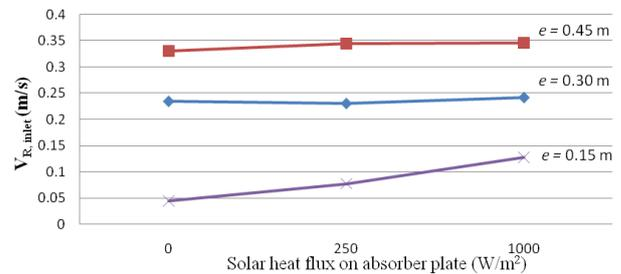
Fig. 8. Variation of room inlet air velocity,  $V_{R,inlet}$  with chimney width,  $e$  (for  $U_\infty = 1$  m/s, and various heat flux on absorber).
