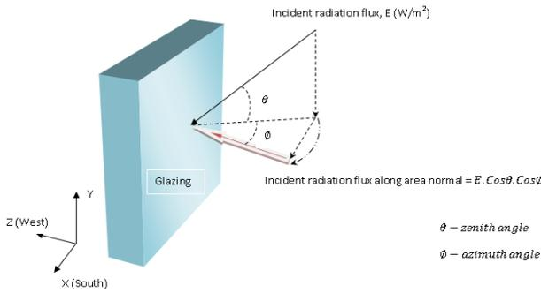
Fig. 9. Calculation of incident (direct) irradiation flux on solar chimney along the area normal.
