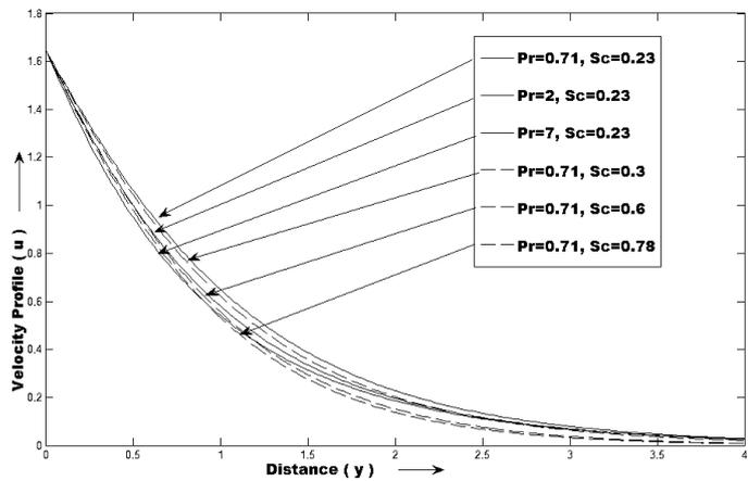
Fig. 2. Effect of Pr and Sc on velocity profile, when  $Gr = 2, Gm = 2, M = 0.5, K = 2, R = 2, S = 2, \alpha = \frac{\pi}{6}, \omega = 1$  and  $t = 0.5$ .
