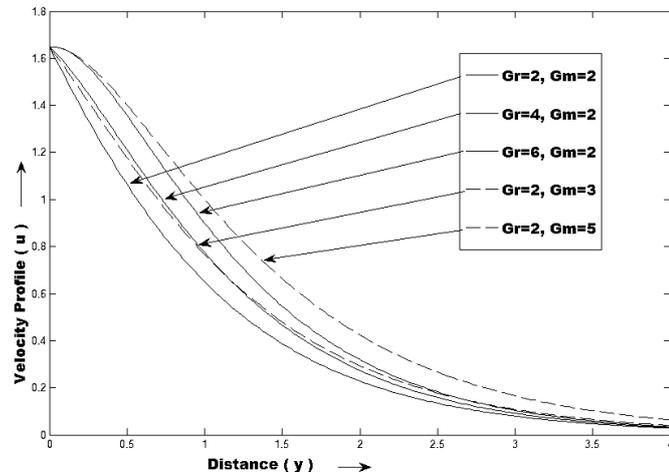
Fig. 3. Effect of Gr and Gm on velocity profile, when  $Sc = 0.23, Pr = 0.71, M = 0.5, K = 2, R = 2, S = 2, \alpha = \frac{\pi}{6}, \omega = 1$  and  $t = 0.5$ .
