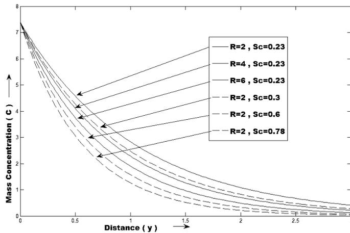
Fig. 7. Effect of R and Sc on Mass Concentration, when  $t = 0.5$ ,  $\omega = 2$ .
