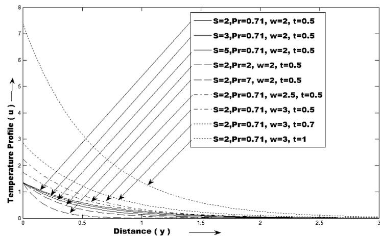
Fig. 6. Effect of S, Pr, t and  $\omega$  on Temperature profile, in the absence of other parameters.
