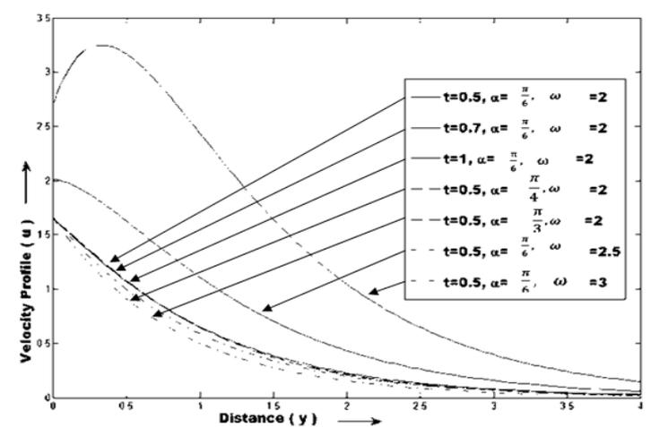
Fig. 5. Effect of  $\alpha, t$  and  $\omega$  on velocity profile, when  $Sc = 0.23, Pr = 0.71, M = 0.5, K = 2, R = 2, S = 2, Gr = 2$  and  $Gm = 2$ .
