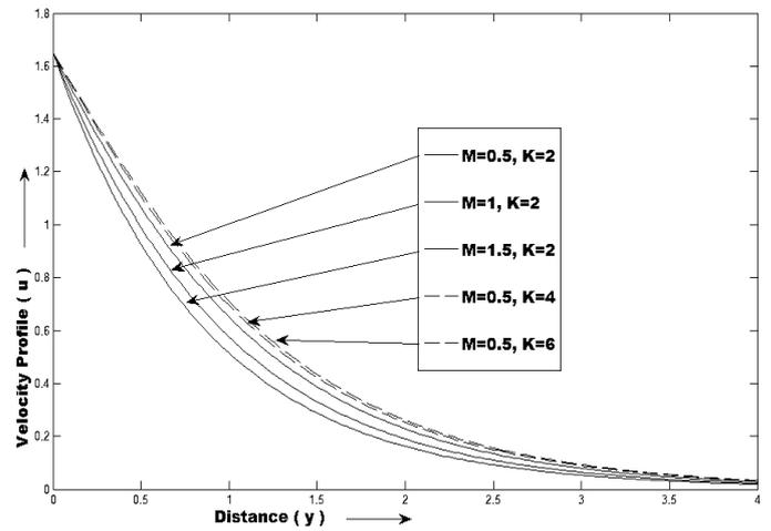
Fig. 4. Effect of M and K on velocity profile, when  $Sc = 0.23, Pr = 0.71, Gr = 2, Gm = 2, R = 2, S = 2, \alpha = \frac{\pi}{6}, \omega = 1$  and  $t = 0.5$ .
