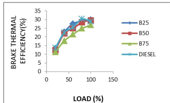
Graph 4.2. Load Vs Brake thermal efficiency at 200 bar & 23° btdc.
