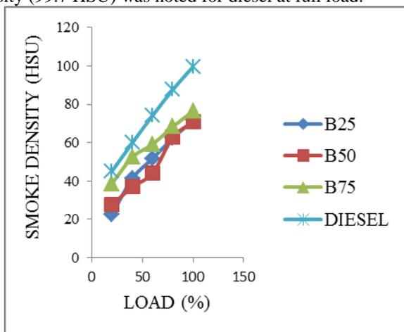
Graph 4.6. Load Vs Smoke density at 200 bar & 23° btdc.
