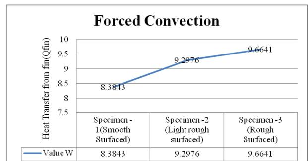
Fig. 6.4. Rate of heat transfer from the fin (Q<sub>fin</sub>) for Forced convection.
