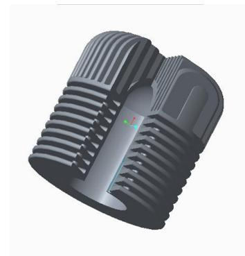
Fig. 2.2. Fin Arrangement of IC Engine.
