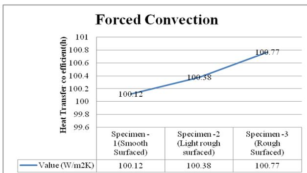
Fig. 6.2. Heat transfer coefficient for Forced convection (h).
