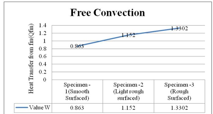
Fig. 6.3. Rate of heat transfer from the fin (Q<sub>fin</sub>) for Free convection.
