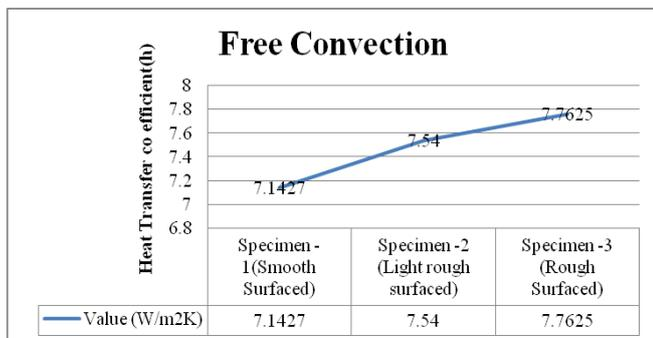
Fig. 6.1. Heat transfer coefficient for Free convection (h).
