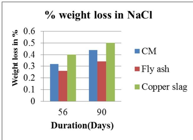
(a). Immersed in sodium chloride solution.
