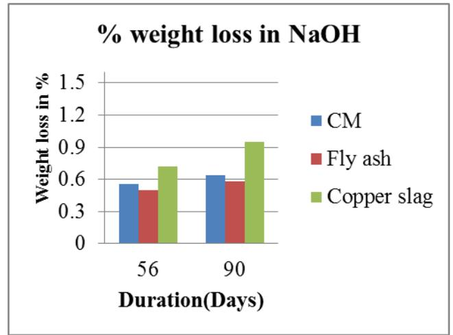
(c). Immersed in alkali solution.
