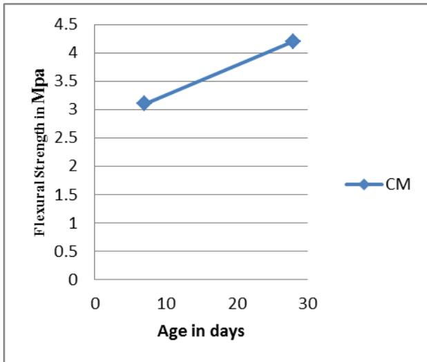
(c). Flexural strength of control mix.
