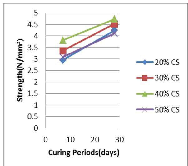
(b). Splitting tensile strength of copper slag.
