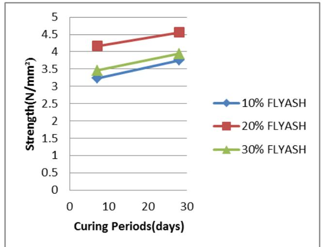
(c). Flexural strength of fly ash.
