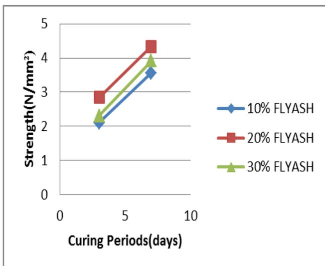
(b). Splitting tensile strength of fly ash.
