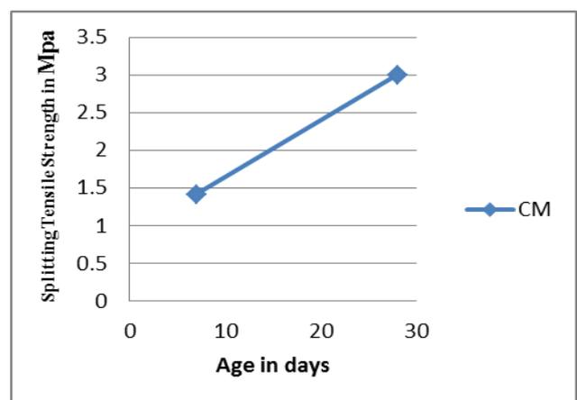
(b). Splitting tensile strength of control mix.
