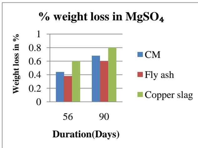
(b). Immersed in magnesium sulphate solution.
