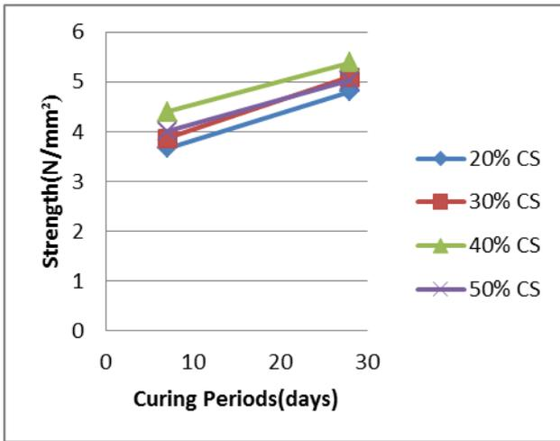
(c). Flexural strength of copper slag.
