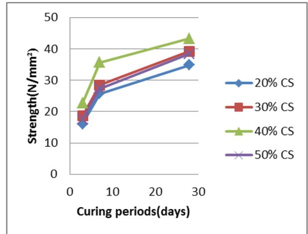
(a). Compressive strength of copper slag.
