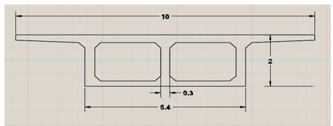
Fig. 1. Cross-sectional details of rectangular box girder (all dimensions are in meter).
