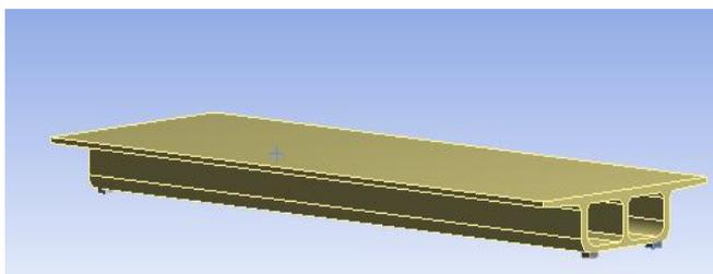
Fig. 8. Perspective view of circular straight box girder.
