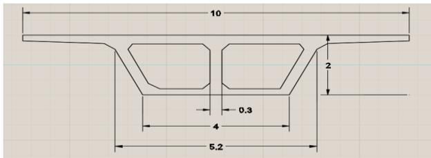
Fig .4. Cross-sectional details of trapezoidal box girder (all dimensions are in meter).
