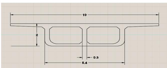
Fig. 7. Cross-sectional details circular straight box girder (all dimensions are in meter).
