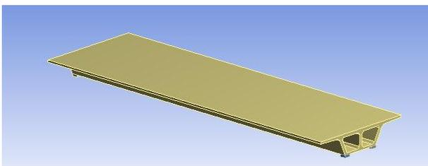
Fig. 5. Perspective view of trapezoidal straight box girder.
