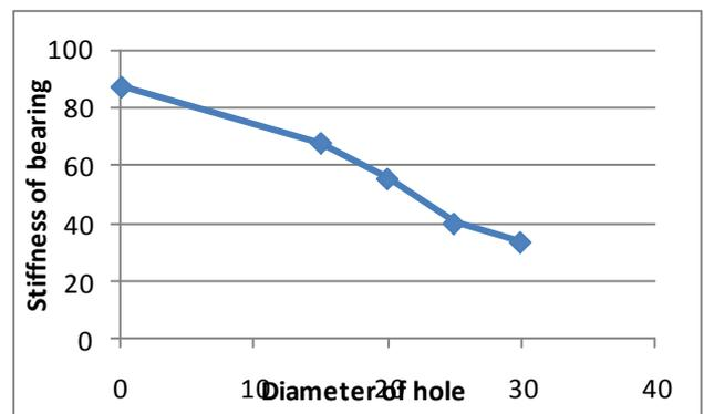
Fig. 6. Variation of stiffness with diameter of hole in the bearing.
