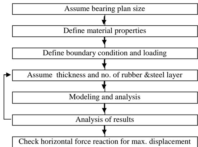
Fig. 2. Design flow chart of bearing.
