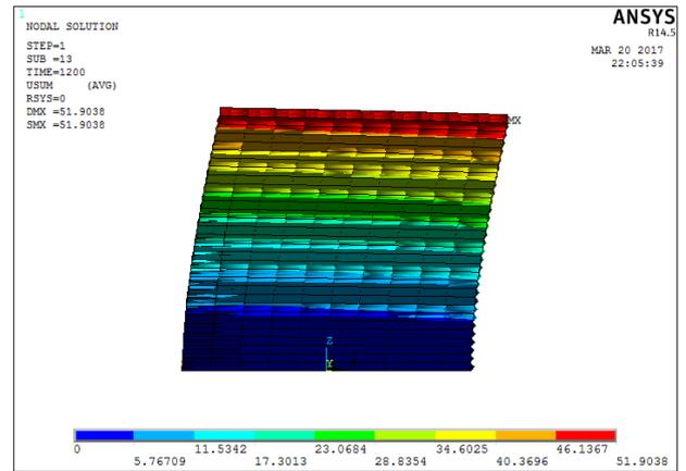
Fig. 5. Deflected shape of bearing without hole.
