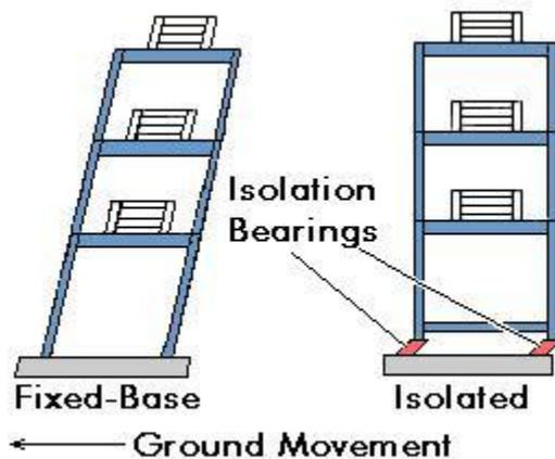
Fig. 1. Basic principle of base isolation.
