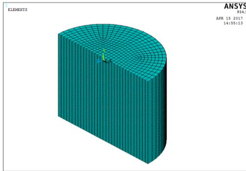
Fig. 7. Model of circular bearing.
