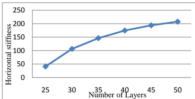
Fig. 11. Variation of stiffness with number of layers.
