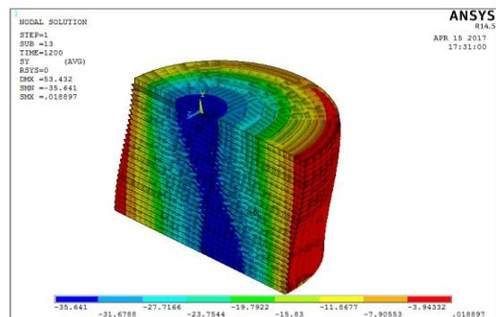
Fig. 10. Vertical stress contour plot – 25 layered.
