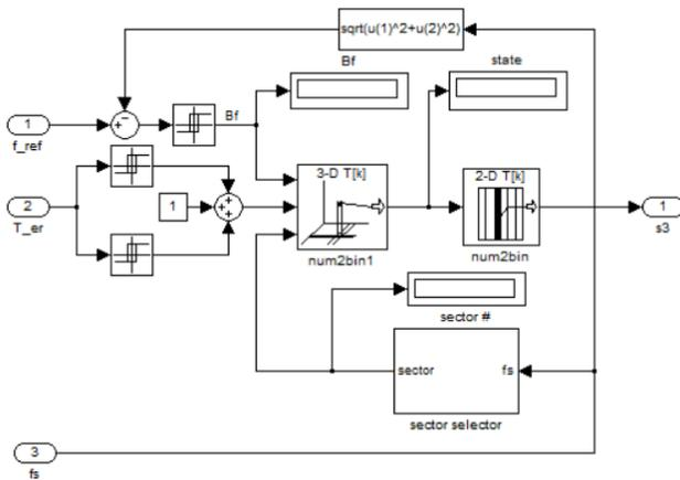
Fig. 3. Stator voltage selector.
