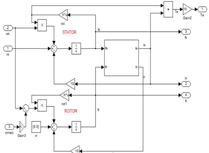
Fig. 4. Modified Induction motor modeling.
