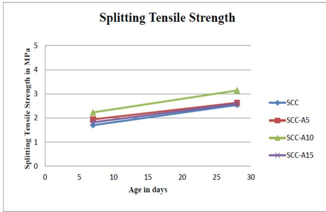
Fig. 4. Graphical representation of split tensile strength of SCC and SCC with Alccofine.
