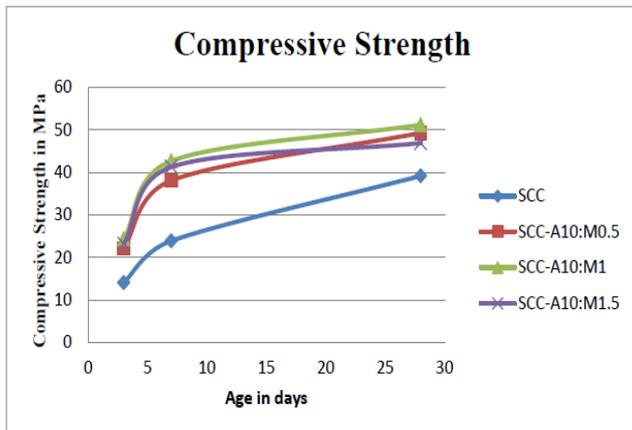
Fig. 5. Graphical representation of compressive strength of SCC and SCC with Optimum Alccofine and Micro steel fiber.
