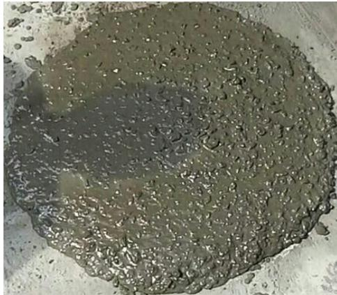
Fig. 1. Slump flow.
