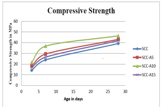
Fig. 2. Graphical representation of compressive strength of SCC and SCC with Alccofine.
