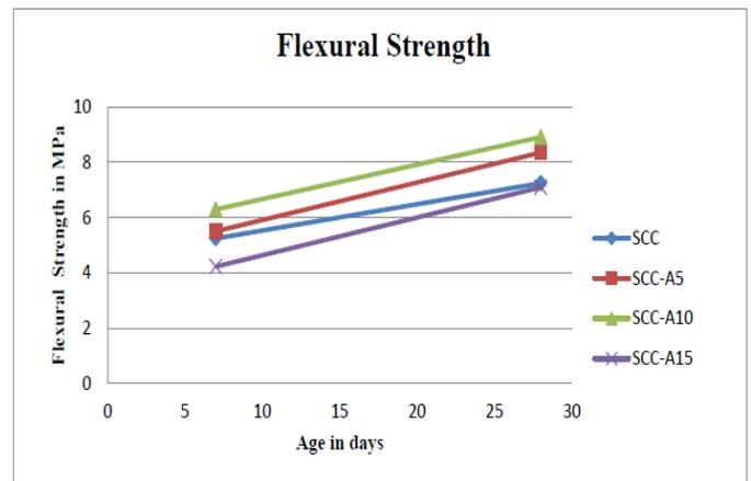
Fig. 3. Graphical representation of flexural strength of SCC and SCC with Alccofine.
