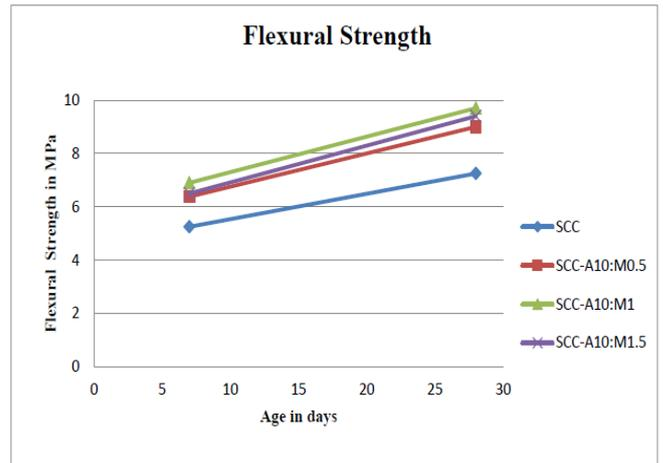
Fig. 7. Graphical representation of flexural strength of SCC and SCC with Optimum Alccofine and micro steel fiber.
