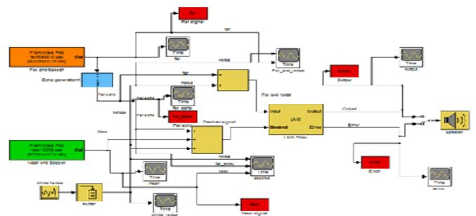
Fig. 1.2 Simulink model of AEC using LMS adaptive filtering
