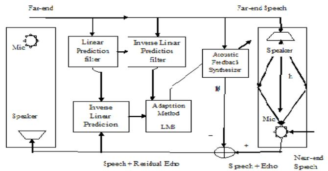
Fig. 1.5. Block diagram of the LMS adaptive AEC with LP filter
