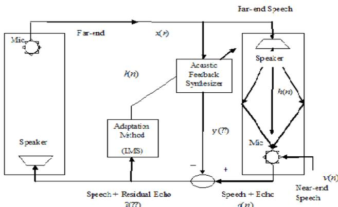
Fig. 1.1 Block diagram of the conventional AEC
