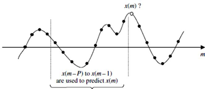
Fig. 1.4. Concept of prediction of the future sample  $x(m)$  from its 'P' past samples
