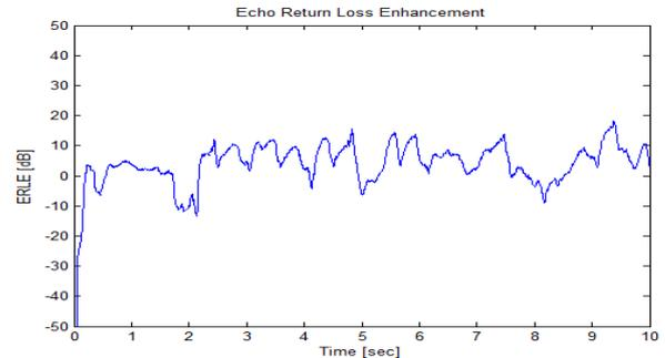
Fig. 1.8 (a). ERLE for LMS adaptive filter
