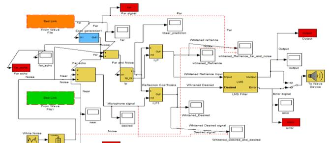
Fig. 1.6. Simulink model of AEC using linear prediction
