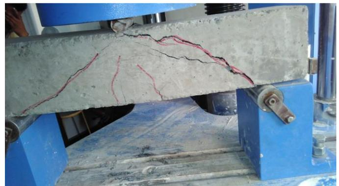
Cracks after applying load
