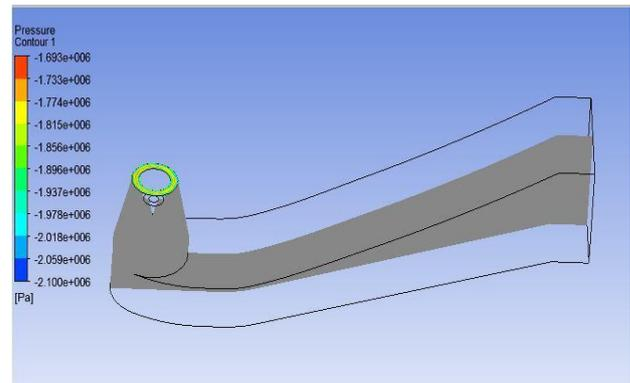
Fig. 3. Pressure at inlet.
