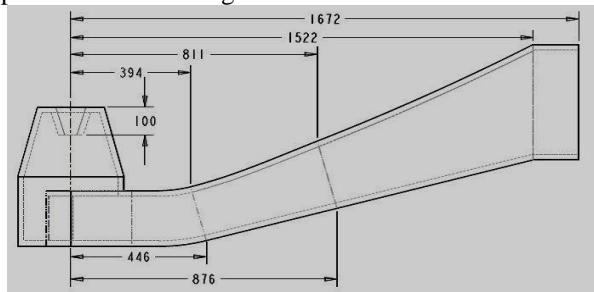
Fig. 1. 2D drawing of draft tube.
