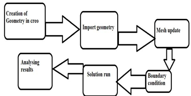
Fig. 6. Steps used in CFD simulation.
