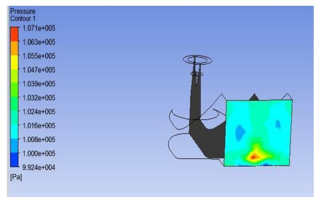
Fig. 4. Pressure at outlet.
