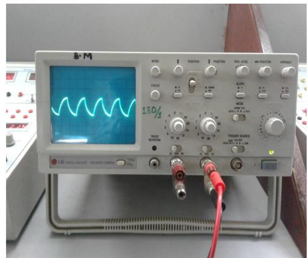
Fig. 8. Capacitor voltage waveform observed on the CRO.
