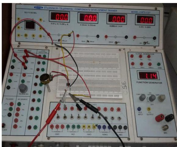
Fig. 6. Photographic view of the system to generate Ramp waveform.
