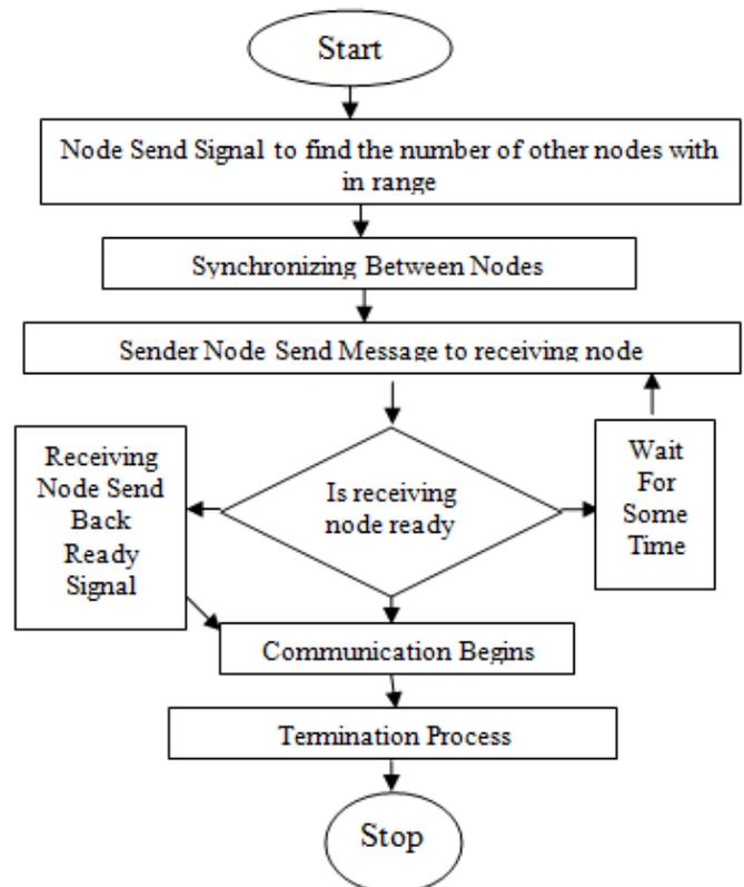
Fig. 1. Working of a general Ad-Hoc network.
