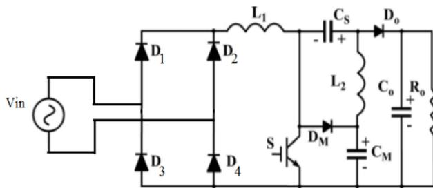
Fig. 3. Modified SEPIC Converter.
