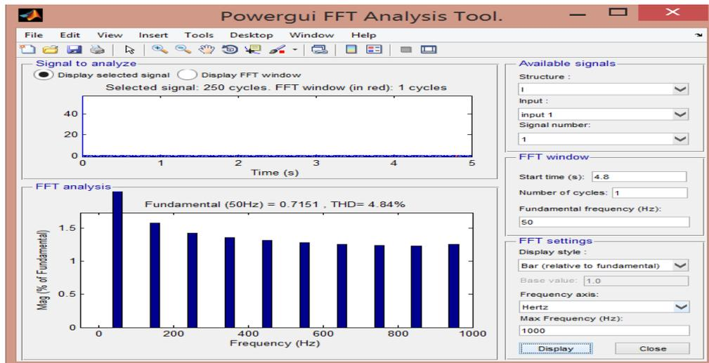
Fig 11. FFT analysis of the modified SEPIC converter with harmonic reduction technique.
