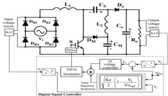
Fig. 7. Block Diagram of pre-regulator.
