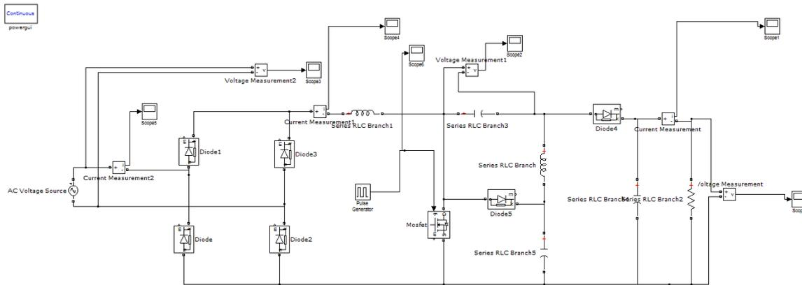
Fig. 8. Matlab simulation of modified SEPIC converter.
