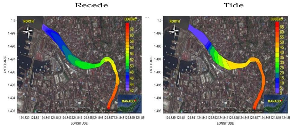
Fig. 2. Flow Velocity Model Map of Tondano River Estuary during the Low Tide and High Tide.
