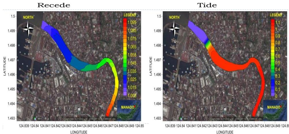
Fig. 3. Model map of transport material dispersion during low tide and high tide in the estuary Tondano river during rainy season.
