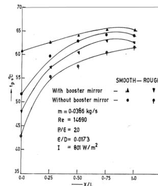
Fig. 4. Plate temperature distribution.
