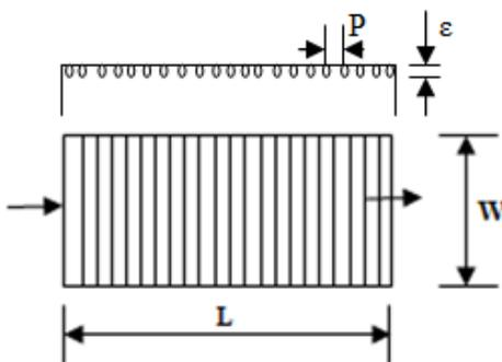
Fig. 2. Absorber plate with artificial roughness.
