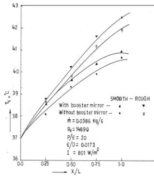
Fig. 5. Air temperature distribution.
