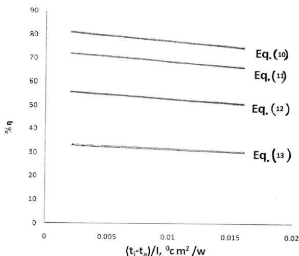
Fig. 11. Thermal performance curves for solar air heaters.
