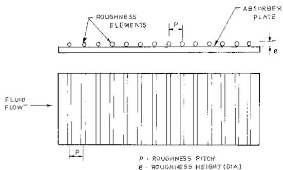
Fig. 3. Roughness distribution on absorber plate as a function of  $p$  and  $e$ .
