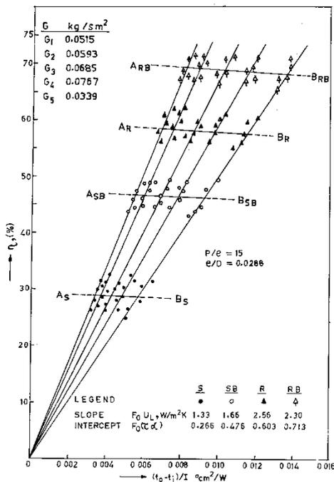
Fig. 8. Performance characteristics of solar air heaters.
