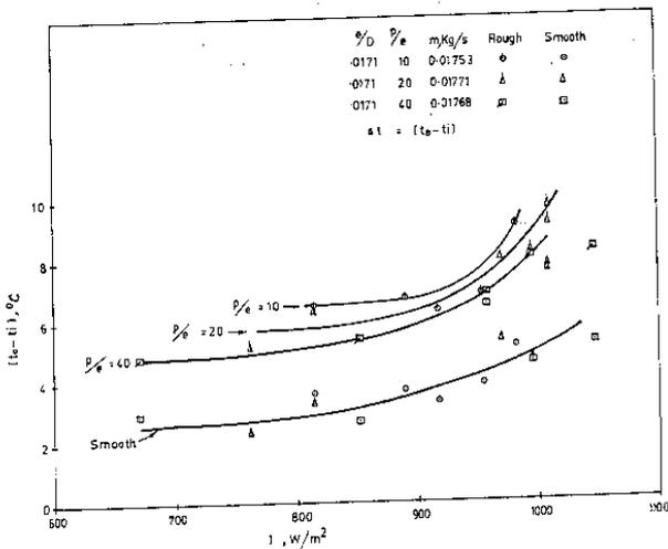
Fig. 1. Air temperature rise as a function of  $p/e$ ,  $e/D$  and  $I$  at almost fixed mass flow rate.
