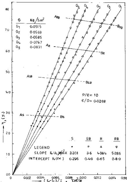
Fig. 7. Performance characteristics of solar air heaters.
