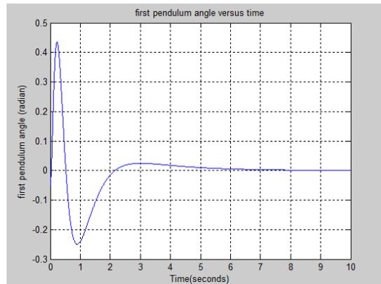
Fig. 2(b). Step response of 1<sup>st</sup> angle.
