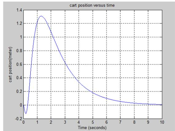
Fig. 2 (a). Step response of cart position.
