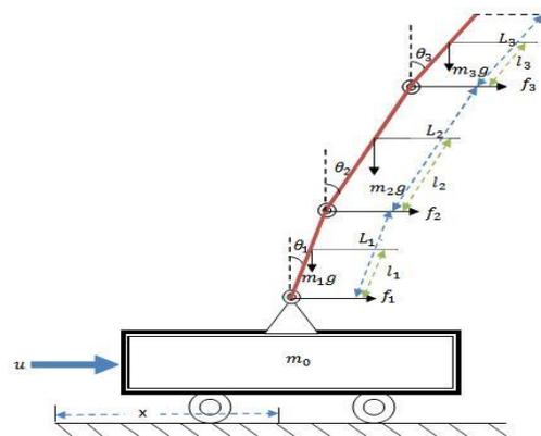
Fig. 1. Schematic of cart TLIP.
