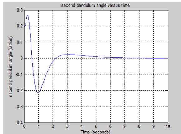
Fig. 2(c). Step response of 2<sup>nd</sup> angle.
