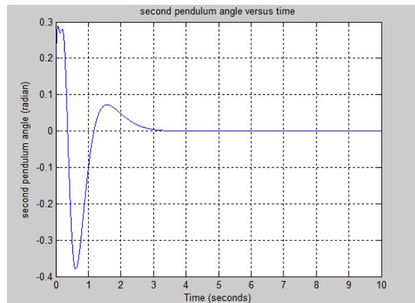
Fig. 3(c): Improved step response of 2<sup>nd</sup> angle.
