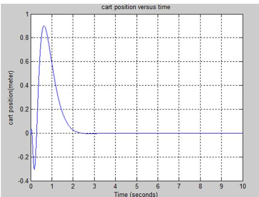
Fig. 3(a). Improved step response of cart position.
