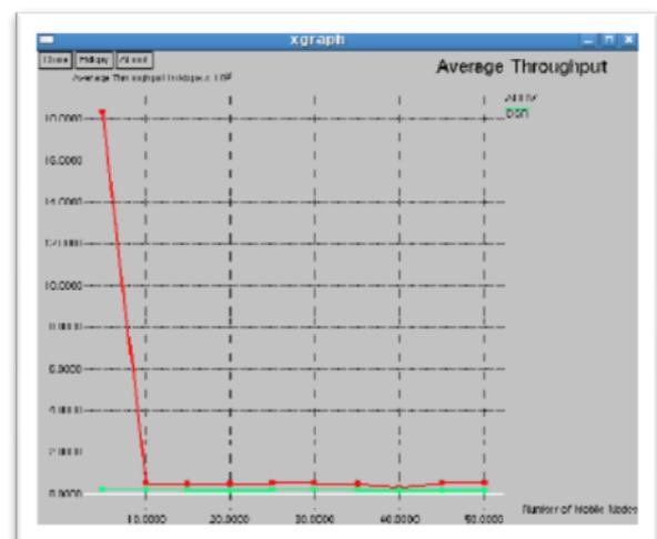
Fig. 3.10. Throughput for AODV and DSR with varying no. of mobile nodes.
