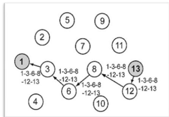
Fig. 2.2. Propagation of the route reply in DSR.
