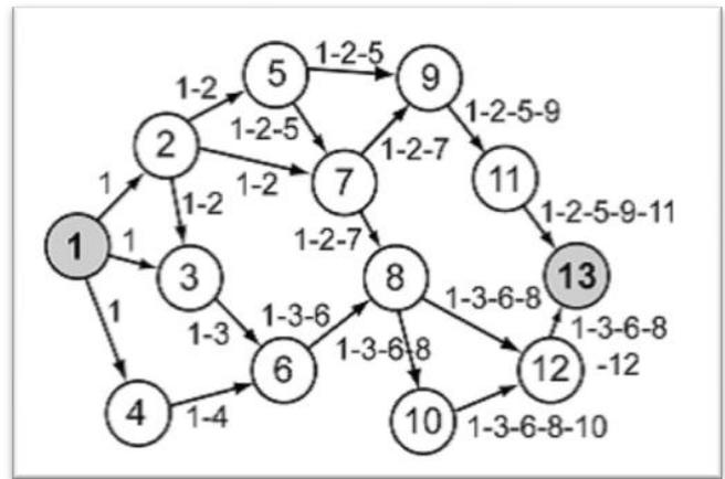
Fig. 2.1. Building of the record during route discovery in DSR.
