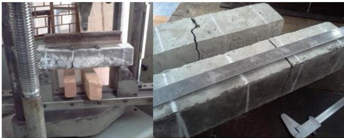
Fig. 3. Flexure Strength Test (a) While testing (b) After testing.
