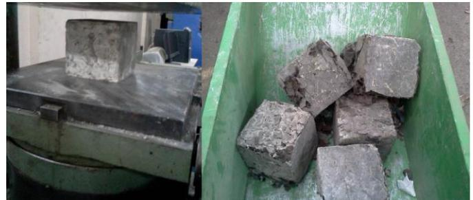
Fig. 2. Compressive Strength Test (a) While testing (b) Crushed cubes.
