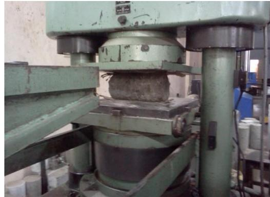
Fig. 4. Splitting tensile strength test.
