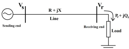
Fig. 1. Single line diagram of a transmission line.
