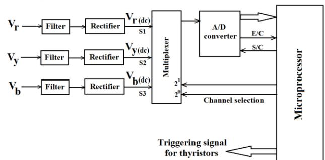
Fig. 4. A schematic diagram of the microprocessor-aided triggering control arrangement for thyristors of TCR-TSC scheme.
