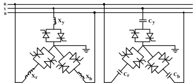
Fig. 3. Three-phase star connected TCR-TSC scheme.
