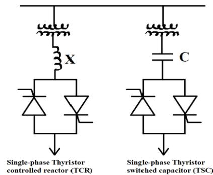
Fig. 2. Thyristor controlled reactor (TCR), thyristor switched capacitor (TSC) scheme.
