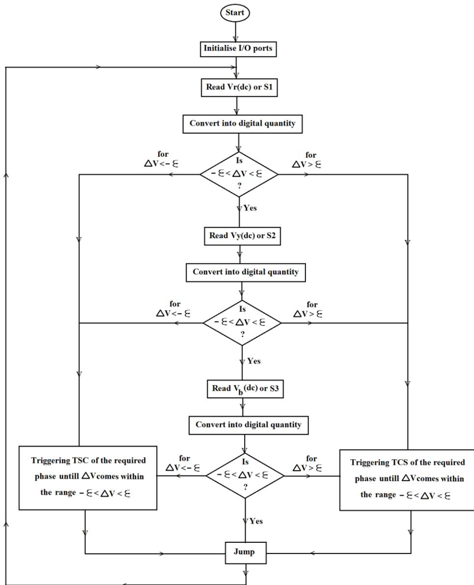
Fig. 5. Flow-chart of the microprocessor-aided voltage stabilizer.
