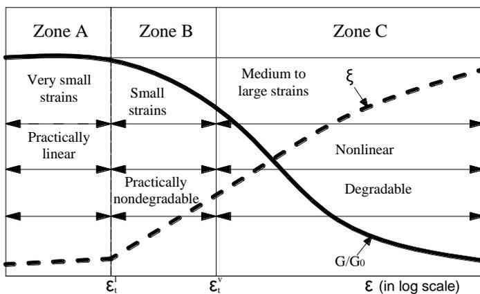
Fig. 5. Typical  $G/G_0$ - $\varepsilon$  and  $\xi$  -  $\varepsilon$  curves proposed by Vucetic [2].
