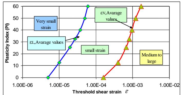
Fig. 6. Relationship between threshold shear strain  $\varepsilon$  and plasticity index PI follow Vucetic, 1994 [2].
