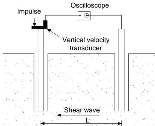
Fig. 13. Cross-hole method of seismic survey.
