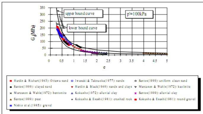
Fig. 2. Relationship between initial shear modulus  $G_0$  as a function of void ratio  $e$  [2].
