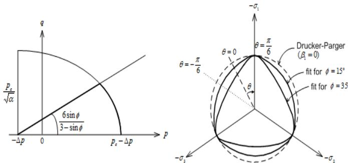
Fig. 12. Hardening soil model in Plaxis 3D.
