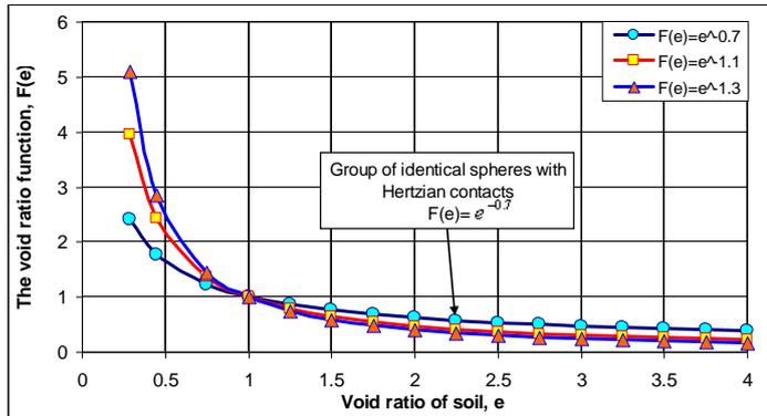
Fig. 1. Curves of relationship between void ratio,  $e$  and function  $F(e)$  with medium of spheres.
