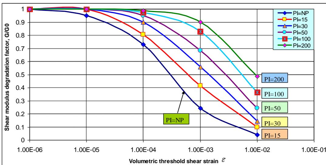
Fig.. 7. Relationship between stiffness degradation factor  $G/G_0$  with threshold shear strain  $\varepsilon$  and IP
