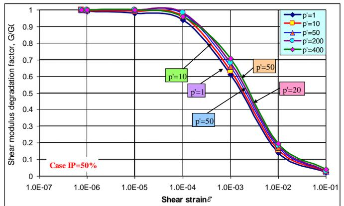
Fig. 8. Relationship between stiffness degradation factor  $G/G_0$  with curves  $\varepsilon - p^*$  (case IP=50% and case IP=NP).
