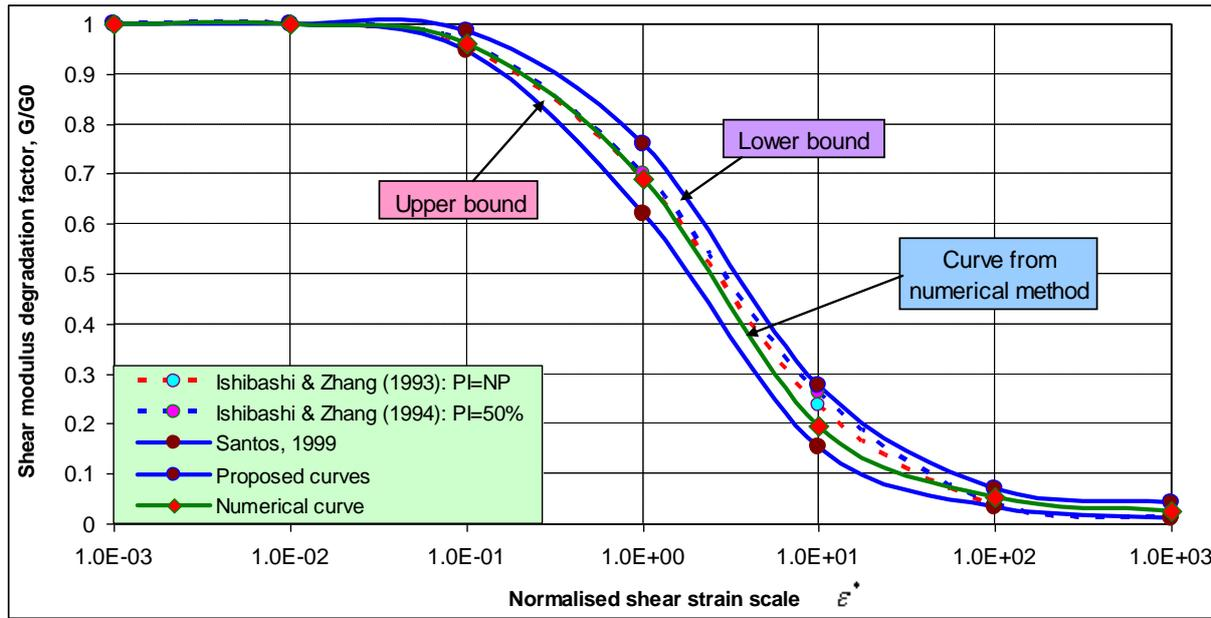
Fig. 11. Proposed stiffness degradation curves and numeral result in  $\epsilon^*$  scale
