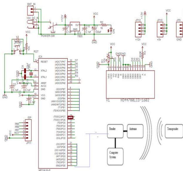
Fig. 3. Circuit diagram.
