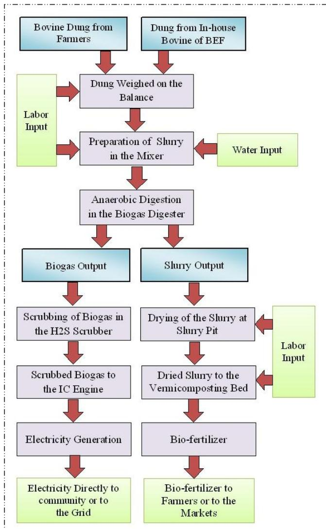
Fig. 1. Layout of proposed bio-energy farm.
