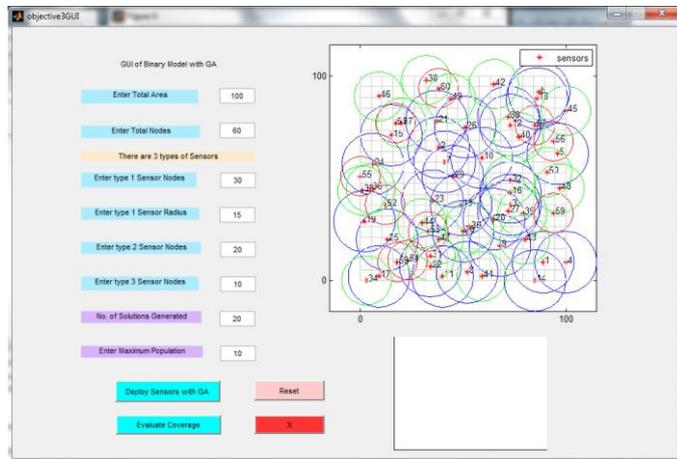
Fig. 3. Snapshot showing the Sensor deployment by binary model using genetic algorithm.
