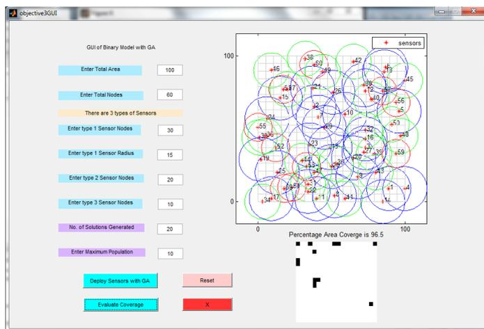
Fig. 4. Snapshot showing the sensor deployment and area coverage by binary detection model using genetic algorithm.
