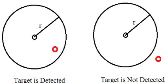
Fig. 1. Detection criteria of binary detection model.
