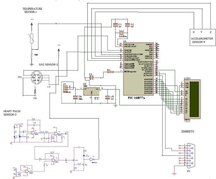
Fig. 1. Circuit of transmitter
