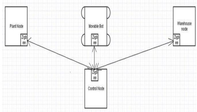
Recommended schematic of the object- handling system
