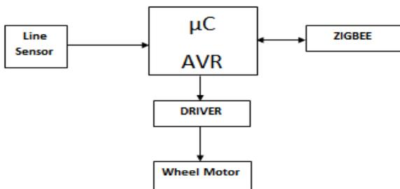
Recommended schematic of the locomotive vehicle
