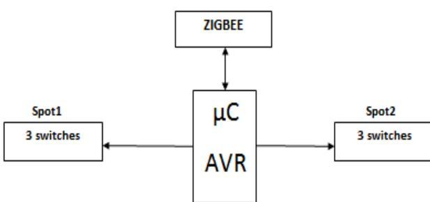
Recommended schematic of the plant node
