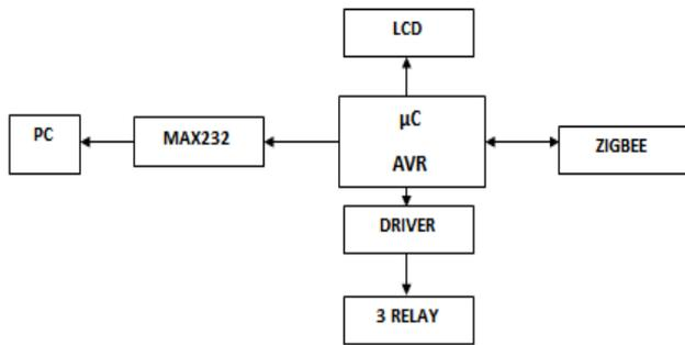
Recommended schematic of the warehouse node
