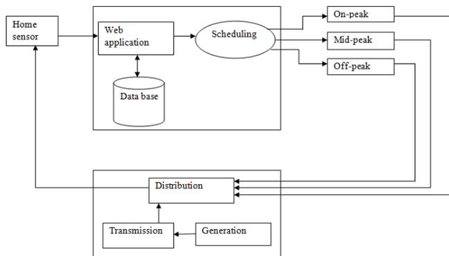
Fig. 1. architecture diagram for the proposed system
