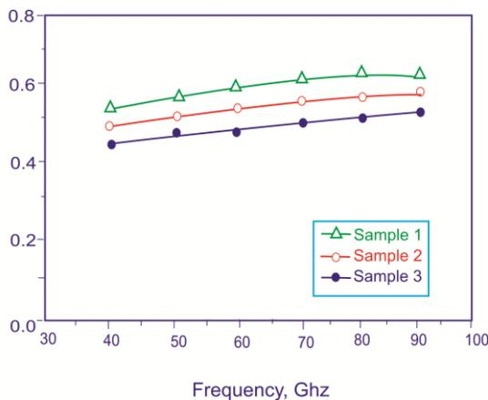
Fig. 3. Variation of transmission coefficient with frequencies
