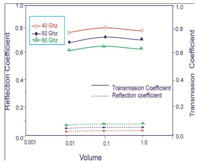
Fig. 6. Variation of reflection and transmission coefficient with volume for different frequencies
