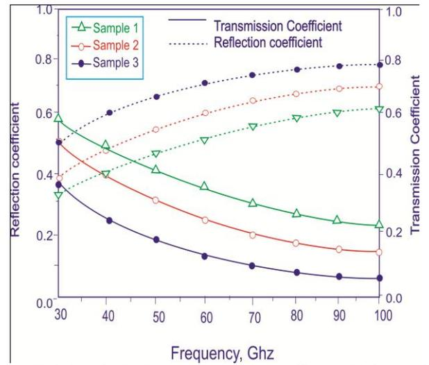
Fig. 4. Variation of reflection and transmission coefficient with frequencies for different sample
