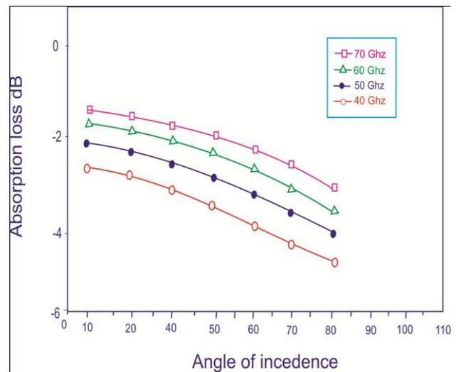
Fig. 9. Variation of absorption loss with angle of incidence for different frequencies
