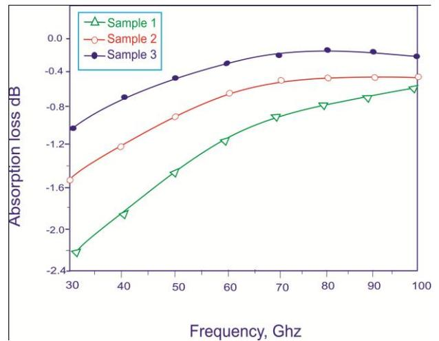
Fig. 5. Variation of Absorption loss with frequency for different sample
