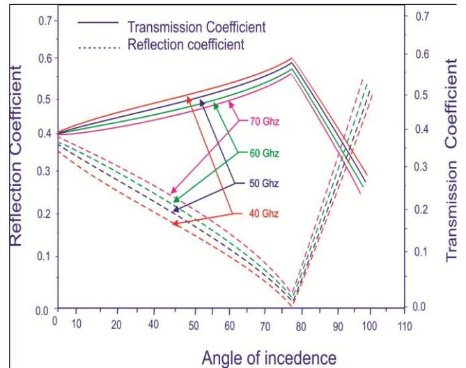
Fig. 8. Variation of transmission and reflection coefficients with angle of incidence for different frequencies (oblique incidence)
