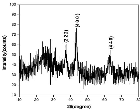
Fig. 2. PXRD pattern of 0.01 M Li doped NiO nanoparticles
