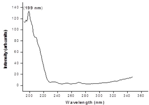
Fig. 7. PL emission spectrum of pure NiO nanoparticles
