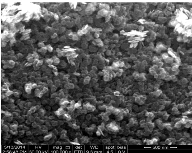
Fig. 6. FESEM image of 0.09 M Li doped NiO nanoparticles with a magnification of 500 nm
