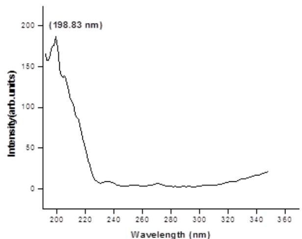
Fig. 9. PL emission spectrum of 0.09 M Li doped NiO nanoparticles
