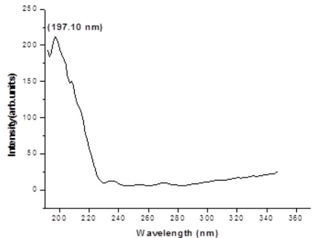
Fig. 8. PL emission spectrum of 0.01 M Li doped NiO nanoparticles
