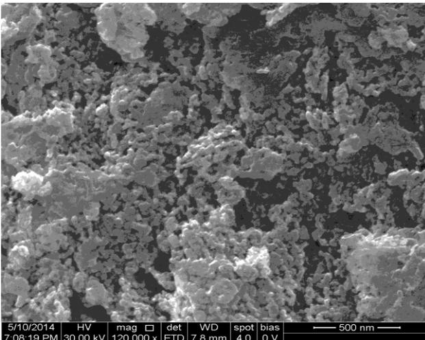
Fig. 5. FESEM image of 0.01 M Li doped NiO nanoparticles with a magnification of 500 nm
