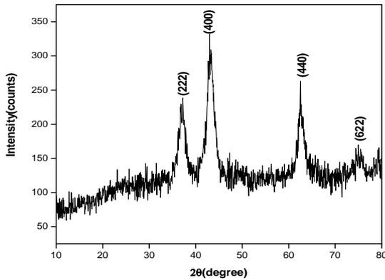
Fig. 1. PXRD pattern of pure NiO nanoparticles
