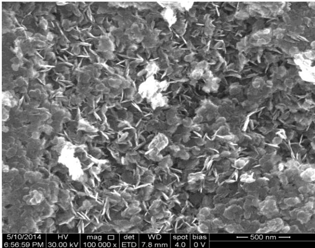
Fig. 4. FESEM image of pure NiO nanoparticles with a magnification of 500 nm
