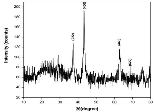
Fig. 3. PXRD pattern of 0.09 M Li doped NiO nanoparticles
