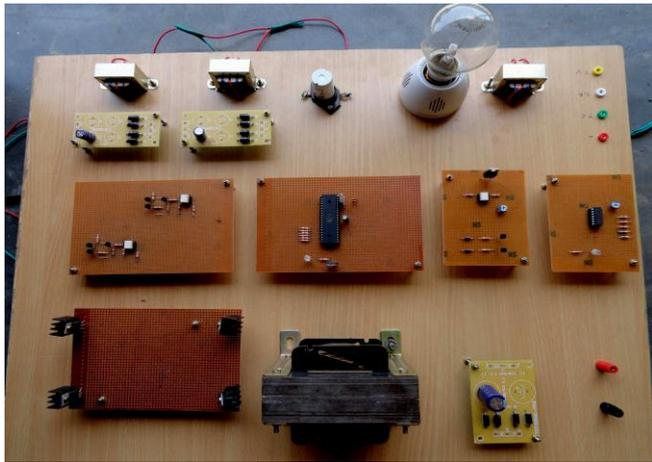
Fig. 13. Hardware module of dynamic voltage restorer (DVR) top view
