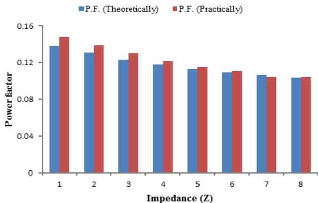
Fig. 4. Calculated the theoretical and practical value of power factor for certain combinations of impedance (LC with resistor 124 Ω).
