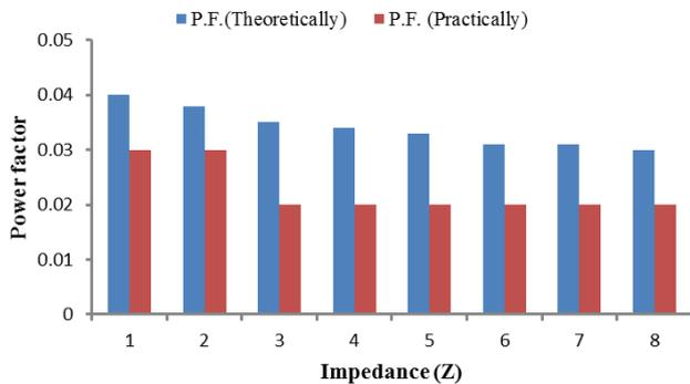
Fig. 3. Theoretical and practical calculated value of power factor for different combinations of impedance (LC with resistor 36 Ω).
