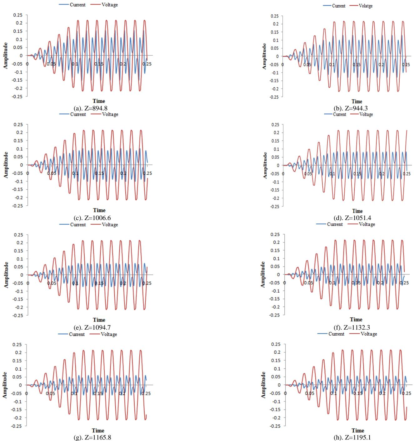
Fig. 2(a-h). Signal for output current and voltage are recorded at 16,000 sampling rate for eight different values of inductance, keeping resistance ( $124\Omega$ ) and capacitor are constant.
