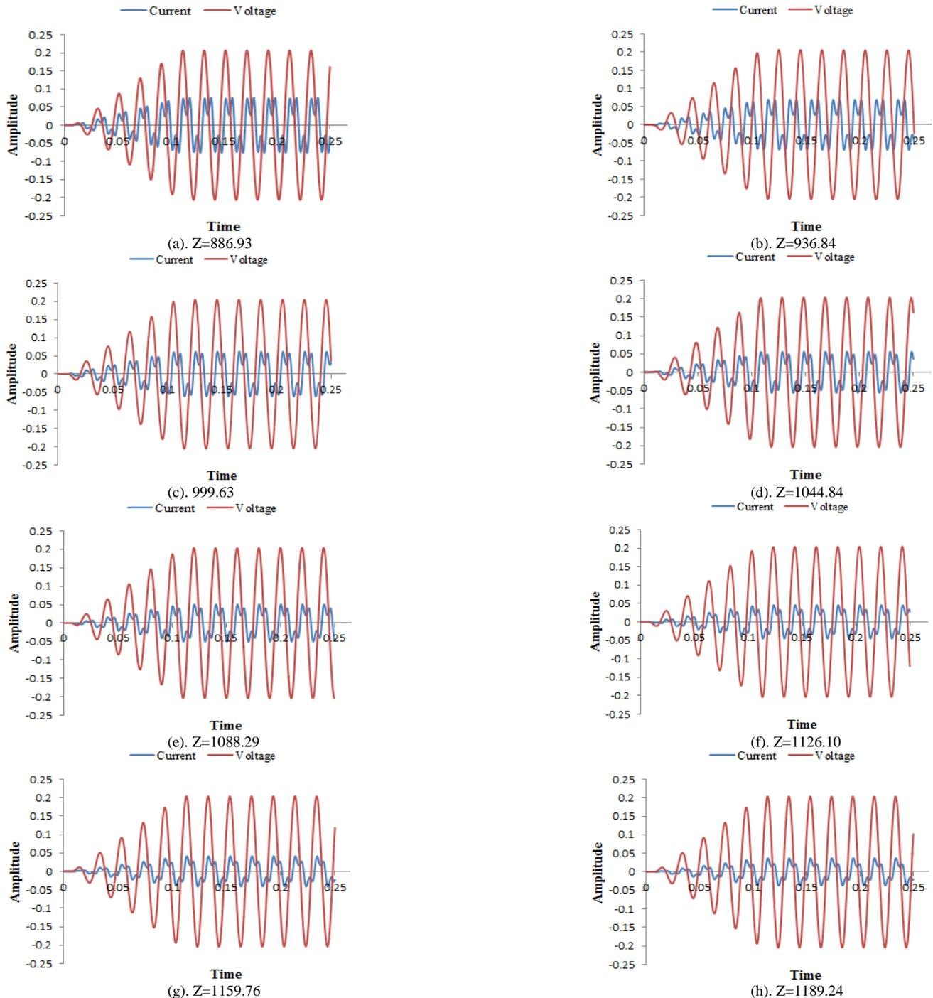
Fig. 1(a-h). Signal for output current and voltage are recorded at 16,000 sampling rate for eight different values of inductance, keeping resistance ( $36\Omega$ ) and capacitor are constant.
